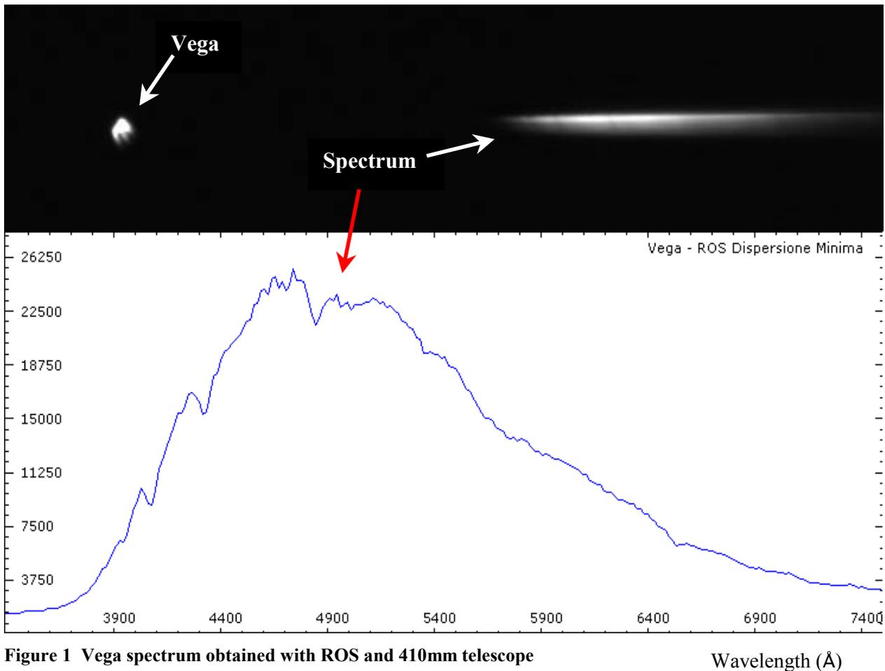
**Figure 1 Vega spectrum obtained with ROS and 410mm telescope**
