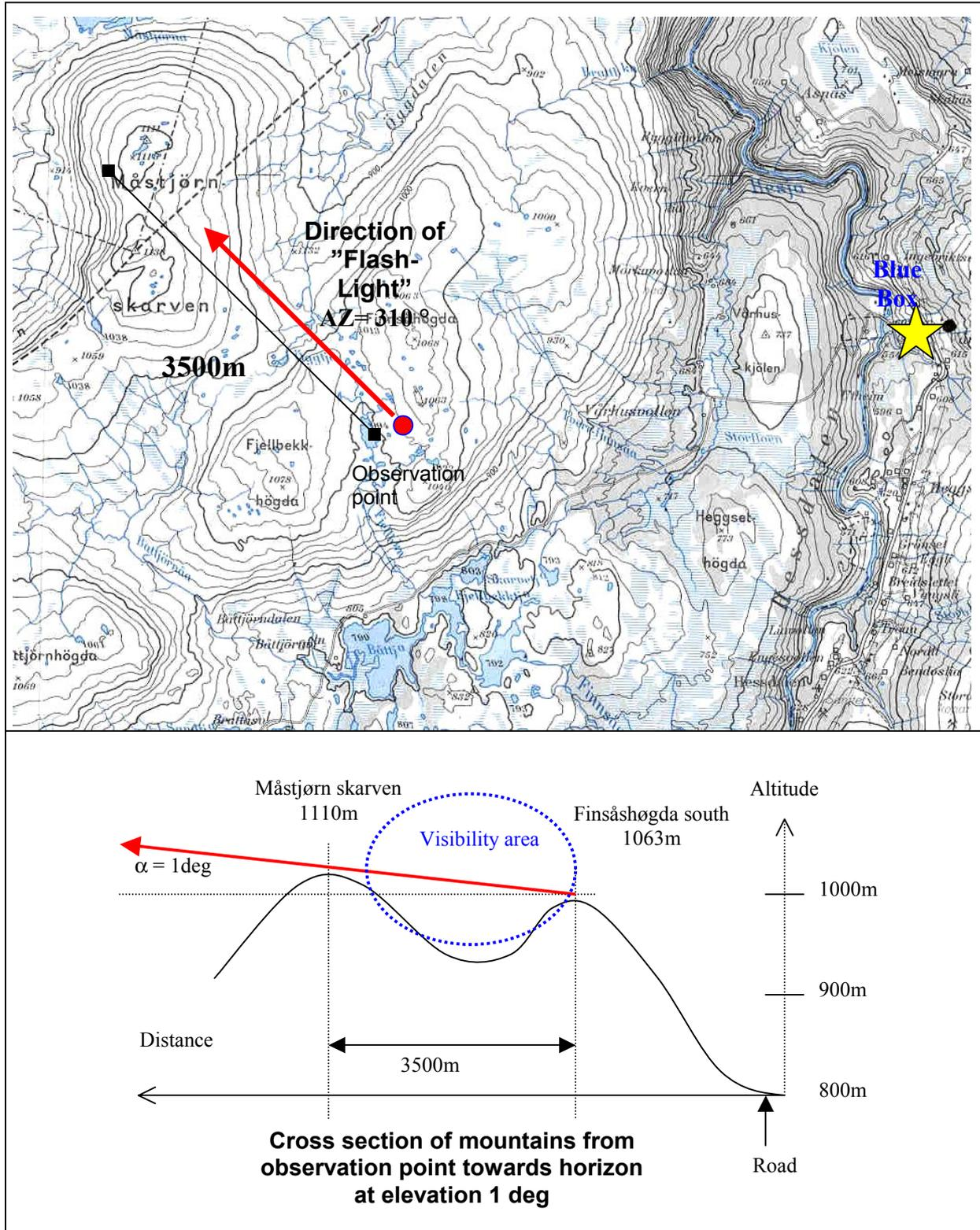
Figure 20. Observation, direction and cross-section analysis of "flash-light" observation. (Survey by B.G. Hauge).
