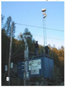
and every time a mysterious light showed up a video recorder started, and a picture was displayed on the Hessdalen internet page. This system was coupled together with a magnetometer, also able to send its data to the internet page. The installed equipment was a combined optical and electromagnetic registration system. The container and the
