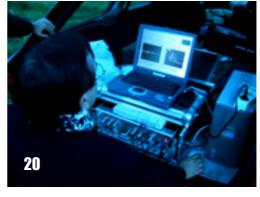
arctic conditions and observations was done from the base camp established at Rogne mountain, where the UHF radar and MPS system was tested out. The MPS system is a transportable TV transmitter and a INSPIRE receiver&transitter. The system is in a small box supplied with batteries and can be left alone on a mountain top for 12 hours. Signals
